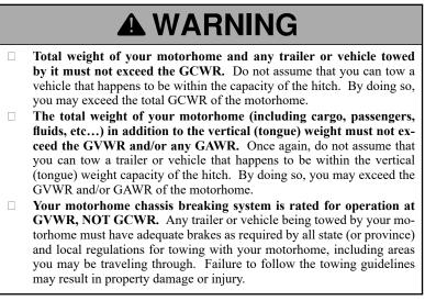
In addition, a separate supplemental braking system must be installed if the towed trailer or vehicle meets or exceeds the minimum weight determined by the chassis manufacturer (this minimum weight rating will vary by chassis and chassis manufacturer).
